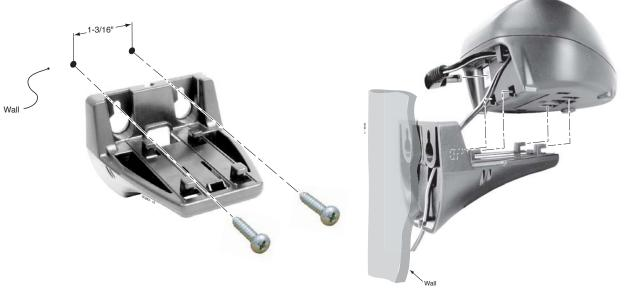
Figure 10: Wall-Mounting the Charger
