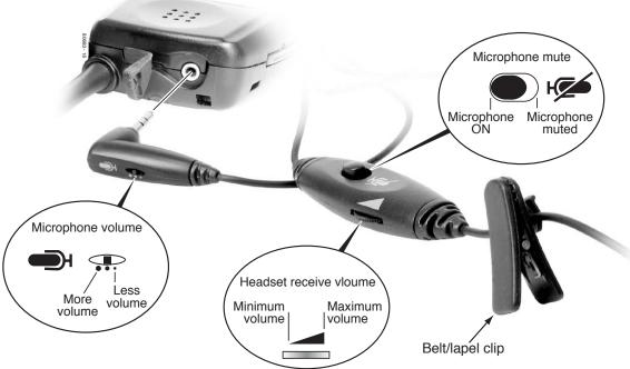
Figure 21: Connecting the Headset and Using the Controls
