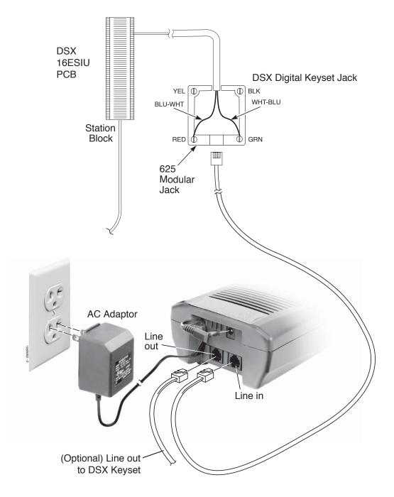
Figure 2: Installing the Base
