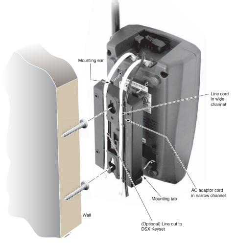
Figure 5: Mounting the Base on the Wall
