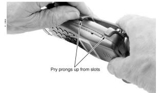
Figure 12: Removing the Belt Clip
