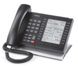
9-line Backlit LCD with 10 programmable buttons
