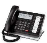
4-line Backlit LCD with 20 programmable buttons
